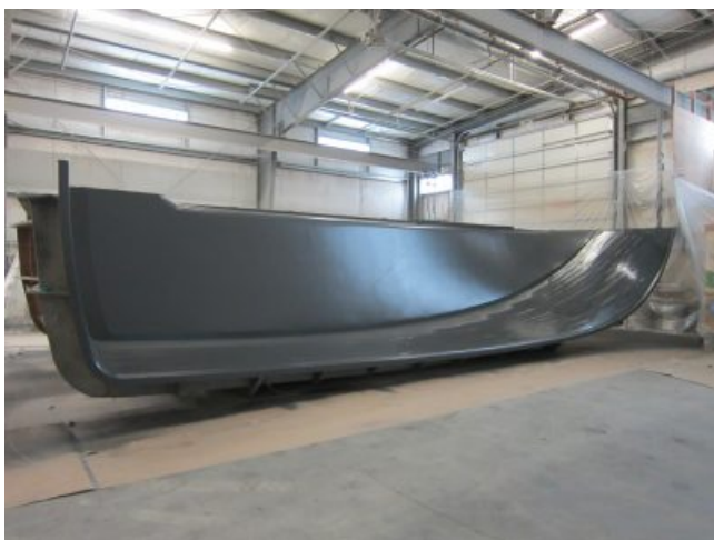
Moulds for hull. They are split then put together to form the entire hull.
